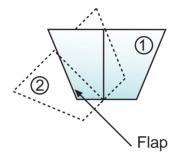
9. Lock the modules in place by folding the flap of unit (1) inside unit (2).
